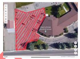
primed; seal coated with a slurry seal, and then lot striped. The cost was \$9,500.00 in 2018. In 2020, when Lindy Roth was Property Director, the west parking lot had 8 areas patched with an unknown process to hold areas together. These are the areas with concentric circles of black asphalt swirled over them. The cost in 2020 was \$2,784.00 and the fix was NOT a good approach as surface is no longer of uniform height in "patched" areas.
